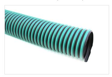
This is a TPRA extraction hose. Manufactured from a thermoplastic rubber and reinforced with a steel spiral helix embedded between two layers. The ducting is designed to be light and very flexible, with good resistance to high temperatures, chemicals, and abrasion.
