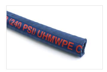
This is a high quality 16 bar chemical suction and delivery hose. The hose is a smooth UHMWPE tube with a protective abrasion and ozone resistant blue EPDM rubber cover.
