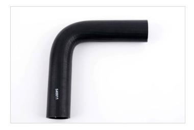
This is a black EPDM rubber 90° elbow, with a polyester reinforcement and great resistance to heat, weather and ageing.
