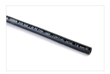
This is a black FKM/NBR rubber fuel hose, specially designed for automotive and engine applications. The hose is suitable for petrol, diesel, ethanol, gasoline, oxidized sour gas, oils and biodiesel. This hose meets SAEJ30R9 standards and is designed to withstand E5 and E10 grades of bio-ethanol enriched petrol formulations.
