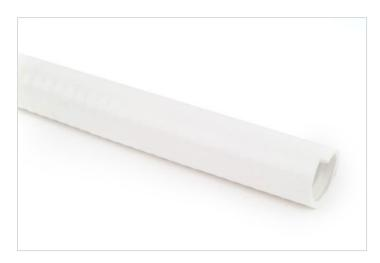
Strong, very flexible and smooth white plasticized PVC hose. This hose is shock resistant and has a galvanised steel spiral reinforcement. Used for suction and discharge for sanitary installation in marine and domestic use.
