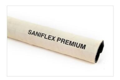
Rubber sanitation hose with a black SBR rubber tube and high tensile synthetic fabric reinforcement. This hose has a white ozone, weather and abrasion resistant SBR rubber cover. Suitable for conveyance of effluent odour free suction and discharge for sanity installations in marine and domestic use with low odour permeability.
