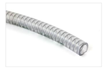
This is a transparent hose produced with a special bio-based compound suitable for the transport of food liquids, beverages, fruit juices, wine and liquors with up to 50% alcohol concentration as well as for the passage of milk and dairy products, according to FDA CFR. 21 (Item 167.170) and Reg. EU 10/2011 (classes A, B, C, D1).
