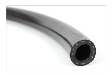
This is an agricultural spray hose, designed for spraying of herbicides, insecticides, and liquid fertilizers. The tube of the hose is a smooth flexible black PVC, which has an outer smooth black PVC cover. The tubing is reinforced with a polyester braid and is suitable for temperature ranging from -15°C to +60°C.
