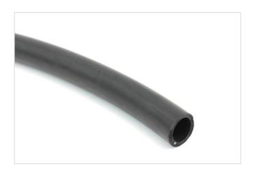
This hose is suitable for oil and fuel up to 40% aromatic content, it is also suitable for some chemicals. It has a smooth extruded black Nitrile rubber tube with a 70 Shore A hardness. The temperature range is -30°C to +125°C.
