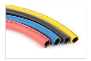
This is a multipurpose air, water and oil hose with a smooth black static conducting NBR synthetic elastomer rubber tube with a coloured SBR/NBR rubber. The hose is reinforced with high tensile textile cords and embedded with an anti-static copper wire. This hose is suitable for the delivery of compressed air, water and oil.
