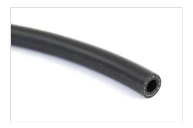
This is a SAE J30 R7 compliant hose, suitable for the delivery of diesel and unleaded petrol in vehicle fuel systems. The tube is manufactured from a fuel and oil resistant smooth synthetic Nitrile rubber, this tube is reinforced with a polyester cord and protected with a smooth black fuel resistant nitrile rubber cover.
