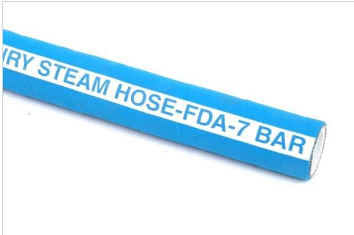
White EPDM food quality, taste and odour free with a high tensile textile cord reinforcement. This hose has a EPDM blue smooth cover with cloth impression. Dairy washdown hose that is resistant against alcohol and bacteria (FDA Approved Material).
