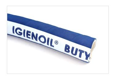
This hose is a liquid food / milk suction & delivery hose. It has a white food quality tube with textile piles and embedded wire helix reinforcement. This hose is FDA approved with BfR recommendations XXI cat. 2, REG CE 1935/04 and 2023/06 DM 21/03/73.
