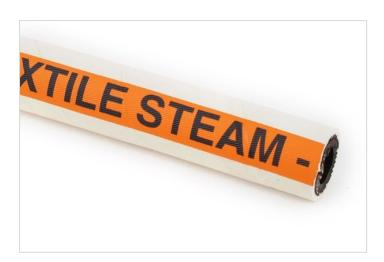
EPDM rubber steam resistant hose with a high tensile synthetic textile reinforcement. This hose has an abrasion, heat, steam, ozone and weather resistant pin pricked special synthetic rubber cover. For saturated steam service when non-marking hose is required.
