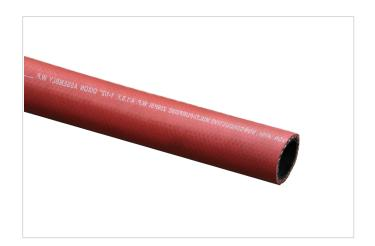
This is a multipurpose air, water and oil hose with a smooth black static conducting NBR synthetic elastomer rubber tube with a red SBR/NBR rubber. The hose is reinforced with high tensile textile cords. This hose is suitable for the delivery of compressed air, water and oil.
