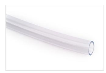
This is a clear PVC unreinforced tubing, made from a USF and DA approved PVC material and suitable for food and drink. The hose has excellent flexibility and transparency and is suitable for conveyance of fluids, gases, powders and granules at low pressure and give withstand temperatures up to  $+60^{\circ}$ C.
