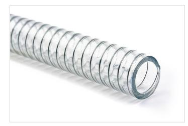
Manufactured carefully from a transparent PVC material, this hose is excellent for general purpose suction and delivery applications. The body is abrasion and ozone resistant and has a smooth bore capable of temperatures of up to 60°C.
